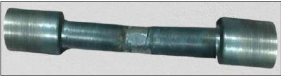
Fig 4: Specimen after welding
